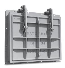
The Waterman Model F-40 Cast Iron Automatic Drainage Gate has a cast iron frame and cover (flap) with machined finished seating surfaces. A minimum  $2\frac{1}{2}$ ° seating angle and double pivoted links assure positive seating.
